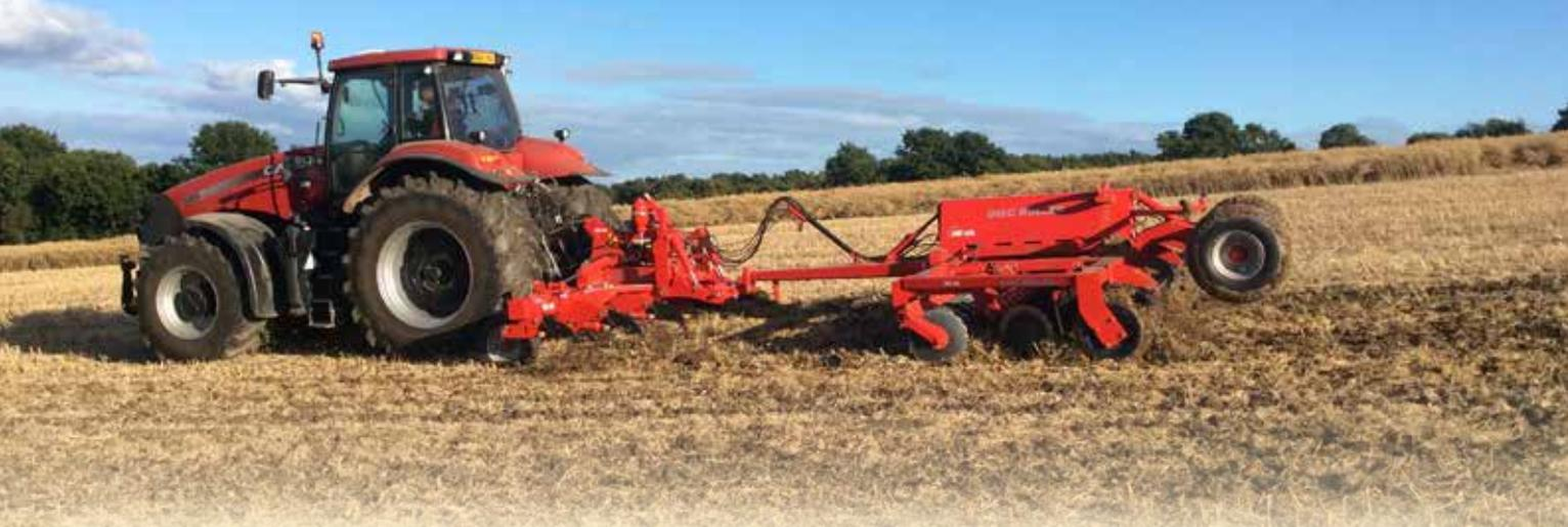
The Combi-Lift Pre-Cultivator fits directly to the tractor linkage and incorporates a rear clevis which can be used to pull a cultivator or drill. Furthermore, the machine can also be fitted with low-disturbance legs to enable light loosening of compaction without heave in mintill or direct drilling situations.
