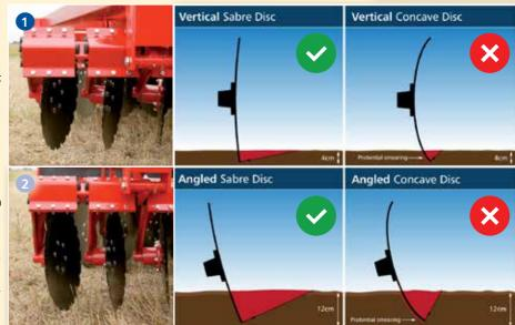
A traditional concave disc or an aggressively angled disc will lift soil and cut out "grooves" but will not move all the soil surface. At the same time it will tend to smear and seal the worked soil creating a disc pan. - DSD
