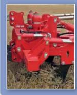
e Combi-Disc's soil loosening legs can be fitted with on the move hydraulic reset. A pressure gauge s the hydraulic system to be set according to the working depth and oil accumulators provide porary expansion room for the hydraulic system when the legs trip. This means that the leg breaks pack quickly and is able to reset immediately once it has passed the obstacle.
