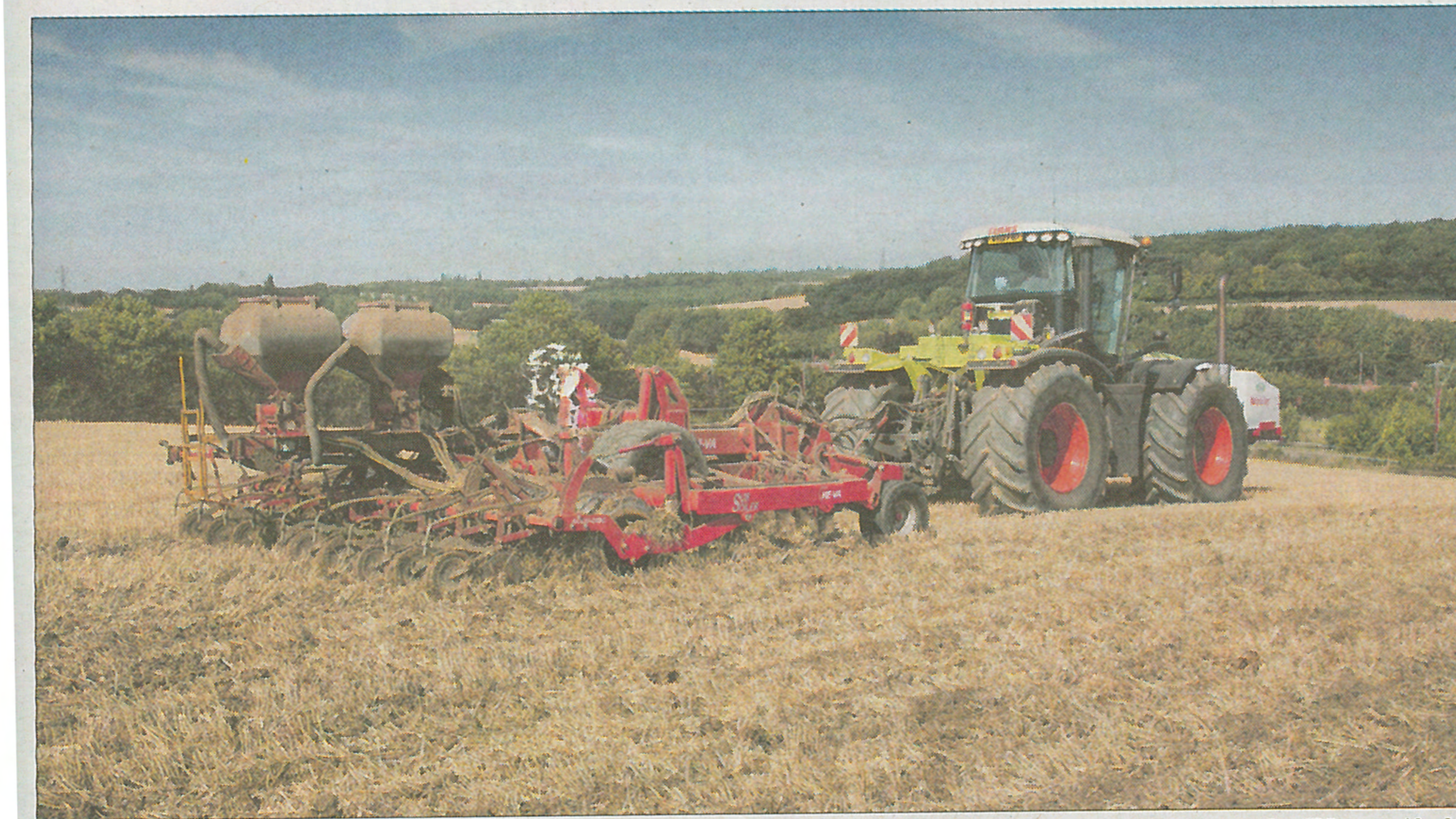
With low disturbance legs, the five-metre He-Va subsoiler and rapeseeding combination establishes up to 40 hectares/day (98 acres/day).
