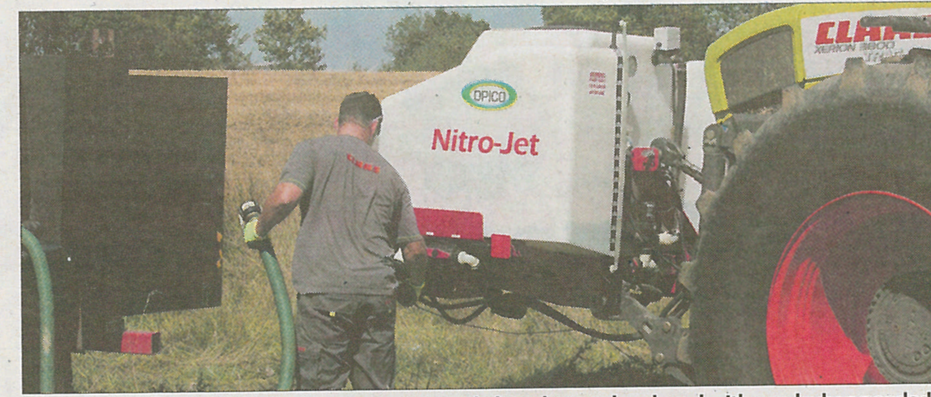
The 1,600-litre Nitro-Jet tank allows nitrogen and phosphate to be placed with seed when needed.
