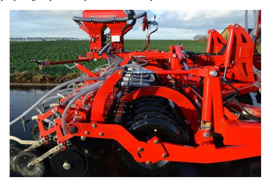
3. Seeding Depth – The Seeding Depth is determined by the relative position of the Press wheel and the Double Disc Coulter. The Press wheel is effectively the Depth control wheel for each Coulter. The Depth is adjusted using the winder which attaches the front mounting bar to the coulter bar. Shorten
