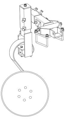
Adjust the edge equipment for the discs in the Combi-Disc so that the excavated soil is collected. Keep the discs away from the ground to avoid bending when turning.
