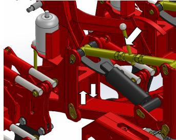
Parallelogram adjustment for depth adjustment.
