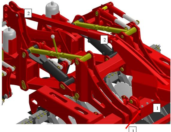
1. Mount the wheel frame bracket and wheel frame on the back of the main frame.
