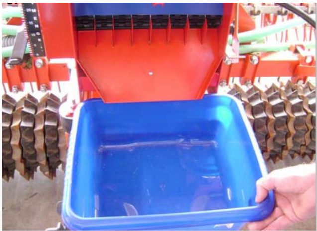
5. Place the calibration trough under the chute
