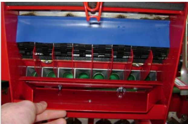
3. Take the chute out, laying beneath the housing
