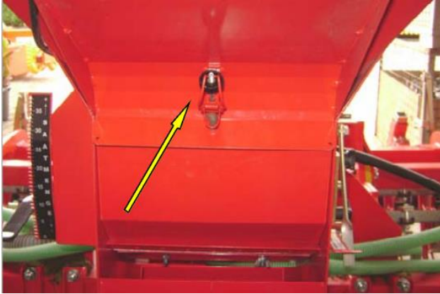
1. Release the cover of the seeder
