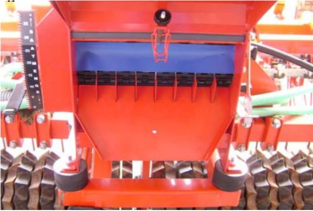
4. Mount the chute under the feed roll
