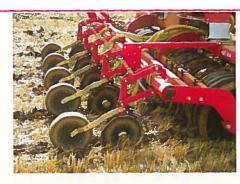
Shown here on a mounted machine, Accu-Disc units combine offset double-disc units and following press wheels.
