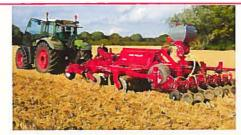
He-Va's Combi-Lift loosener is followed by Disc-Roller cultivating discs, placed in work where needed, with Accu-Disc units at the rear.
