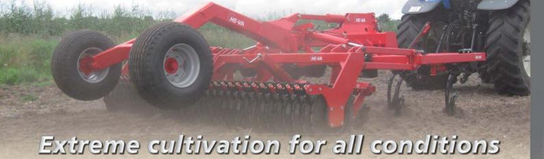
With working widths of 3m, 3.5m, 4m and 5m there is a Triple Tiller to suit the tractor you have.
