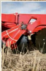
The unique DSD technology is in the way that the aggressiveness of the discs changes with the working depth. When the operator needs the machine to work deeper, the tractor hydraulics are used to alter the working depth of the discs. This is beneficial in two ways, it transfers more weight to the discs but more importantly changes the angle of the disc in its approach to the work producing a more aggressive action which effectively pulls the discs into the soil.
