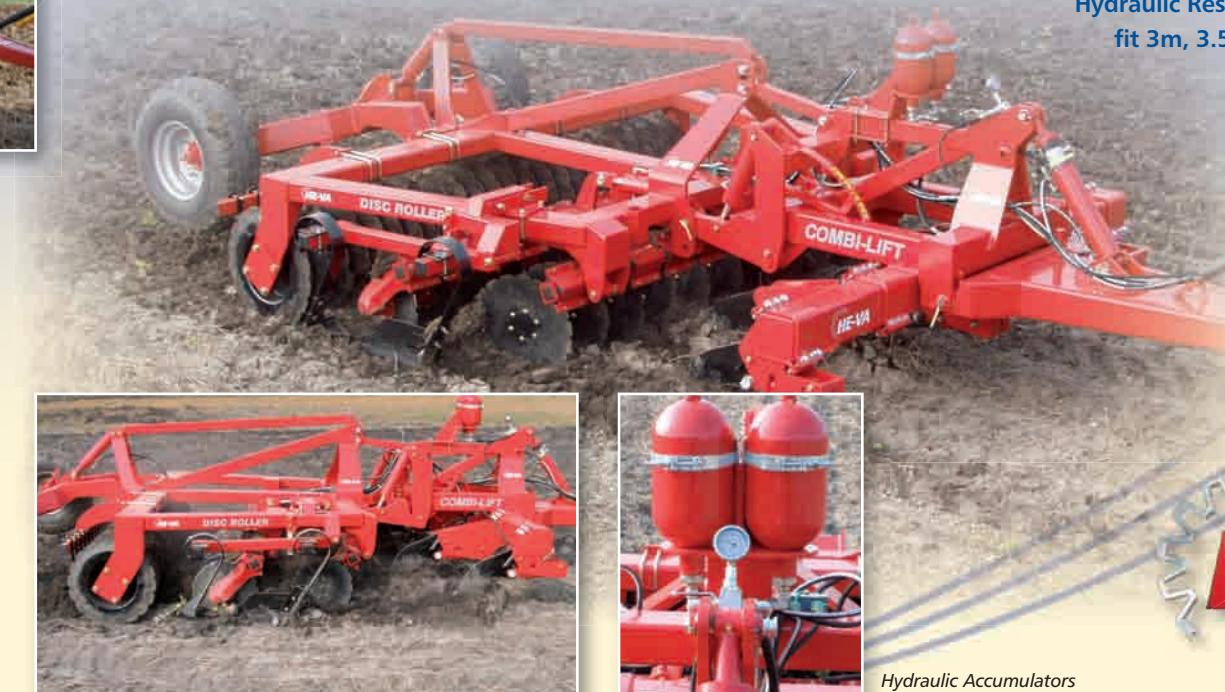
Only available as a trailed unit the Hydraulic Reset Combi-Lift is designed to fit 3m, 3.5m 4m, and 5m Disc Rollers.
