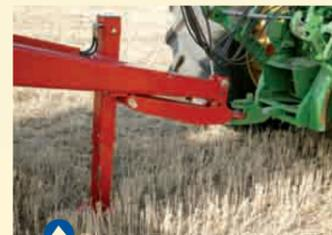
Drawbar height is hydraulically adjustable to suit tractor hitch Trailed 3m, 3.5m, 4m and 5m machines
