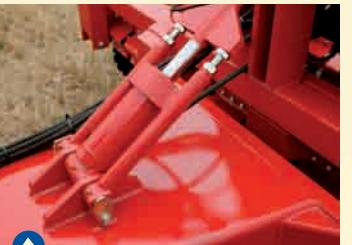
Drawbar height is hydraulically adjustable to suit tractor hitch
