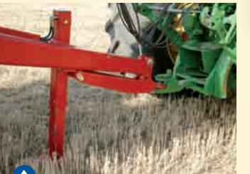
Drawbar height is hydraulically adjusted to suit tractor hitch
