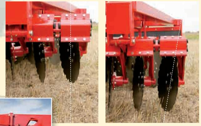
The unique DSD technology is in the way that the aggressiveness of the discs changes with the working depth. When the operator needs the machine to work deeper, the tractor hydraulics are used to alter the working depth of the discs. This is beneficial in two ways, it transfers more
