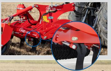
All models are available with hydraulic auto reset for extremely stony conditions. An individual hydraulic cylinder on each leg which is connected to a gas accumulator allows the leg to break back and reset if it comes into contact with an unmovable object.
