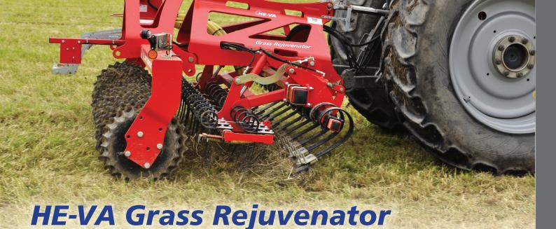
A grassland improvement machine which consists of an aggressive Shattaboard with slicing plates, 2 rows of heavy duty harrow tines, an Air 8 (2.9m, 4.5m models) or an Air 16 grass seeder (6.3m, 8.2m models) and a Prisma roller. The slicing plates and harrow tines break up and level the soil surface in front of the grass seed outlets and the soil is then firmed behind by the Prisma roller. The Grass Rejuvenator comes in four working widths, 2.9m, 4.5m, 6.3m and 8.2m
