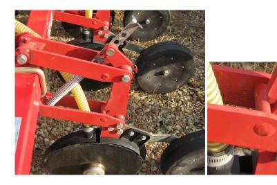
2. It is necessary to set the working height of the mounting bar each parallelogram is fitted to and therefore position of the above pin between the stops. On Trailed Hydraulic Folding machines this is set by adjusting the pairs of Top links shown in the pictures below.
