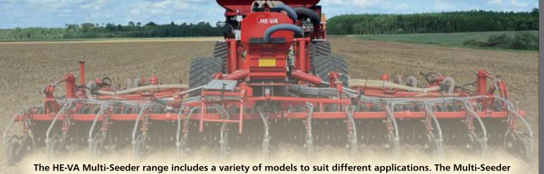
is commonly used to apply grass seed, oilseed rape and slug pellets but can be used to apply many other small seeds and granules. HE-VA have developed bespoke fitting kits to suit the majority of cultivators and rollers ensuring that the operation of neither the host machine or seeder are compromised. Furthermore the Multi-Seeder Twin offers the ability to apply two different products at the same time controlled by a single control box in the cab.
