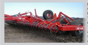
By mounting a Spring-Board in front of the Euro-Tiller harrow, the field is perfectly levelled and the major clods are broken.
