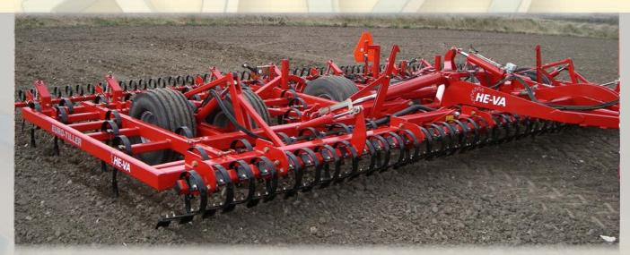
Euro-Tiller models are designed for seedbed preparation on all soil types. The standard harrow has a solid 6 row frame in 60x60x5 cm sectional tubes. With the wide range of extra equipment, the Euro-Tiller can be constructed individually adapted for any farm and soil type. The harrow has the necessary weight and is equpped with all the necessary tools to obtain a perfect seedbed for grain, beets, maize, potatoes and other special crops.
