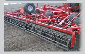
A flat bar roller ø400 mm mounted with the long finger harrow in front leaves a pulverized and light consolidated surface. With its construction of 8 x 40 mm flat steel, this type of roller ensures a perfect soil structure.
